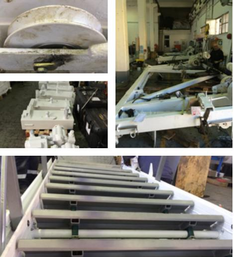
Overhauls of the hydraulic and electrical systems, electrical motors, winches and sheaves. Valves are also replaced and calibrated as per original designs.
